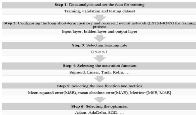
**<Fig. 2> Design process of the LSTM-RNN model**
