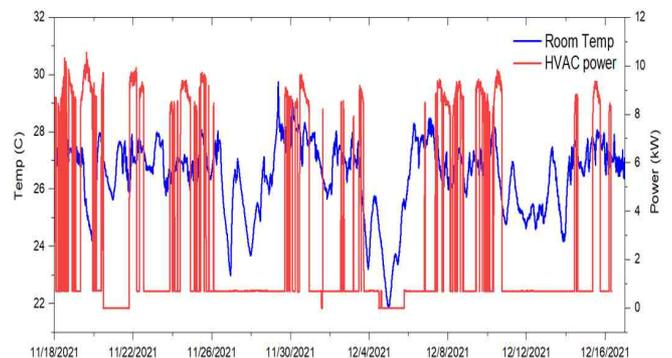
**<Fig. 1> Relationship between the room temperature data and the power demand of an HVAC system**
